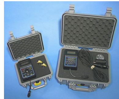
Left - Pelican 1200 carrying case with a 2100 Indicator and two rotor assemblies.
